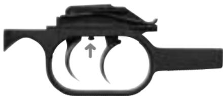
The models of the series 1700 ST are equipped with a double set hunting trigger. The purpose of this trigger is to fire the shot with a minimum of trigger pressure (hair trigger). The double set trigger is operated as follows:
