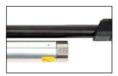
TO SCREW IT OUT: Screw the compressed air cylinder manually approx. 1 turn counter-clockwise.
