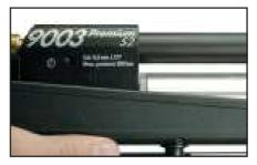
Repeat this process once or twice to allow the air which is still in the rifle to escape. Thus the compressed air cylinder can be screwed out without any pressure on the o-ring.
