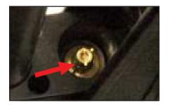
Check the o-ring for any damage.
