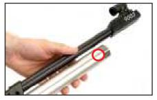
Refer to the drill hole of the compressed air cylinder.
