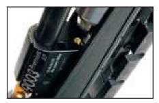
Screw out the compressed air cylinder completely.
