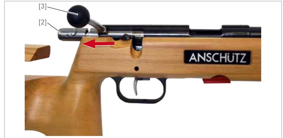
Fig.3 Opening the breech
