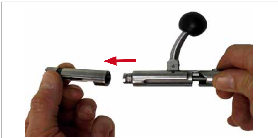
Fig. 16 Pulling off the bolt head
